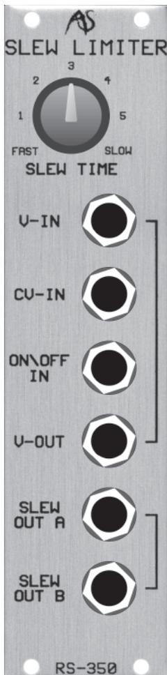
A Slew Limiter - also called a "Lag Processor" - is an example of a voltage processor. It produces no signal of its own, but affects those presented to its input.
