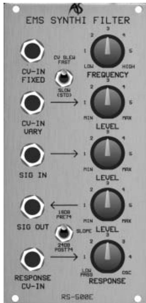
Happily, you don't have to choose between one or the other when configuring your RS Integrator. The RS500E offers both filter characteristics, selectable using a simple front-panel switch.
