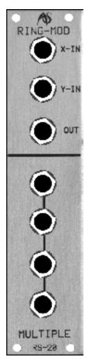
The RS20 contains two independent modules: a high quality ring modulator, and a four-part multiple.
